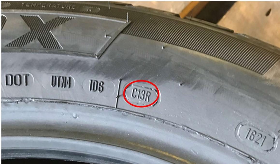
Only tires that exhibit the noncompliant (missing) date code, are being recalled. Tires from DOT weeks 1321 through 1621 that exhibit a compliant date code portion of the TIN are not subject tires and are not eligible for free replacement.
